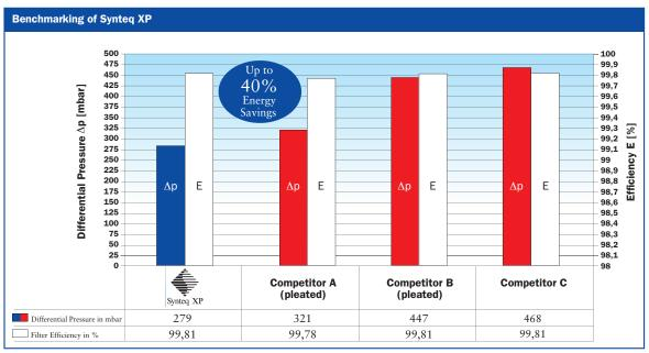
Differential pressure  $(\Delta p)$  and retention rate (efficiency) according to ISO 12500-1, comparable coalescence filter under oil-moistured conditions at 8 bar.
